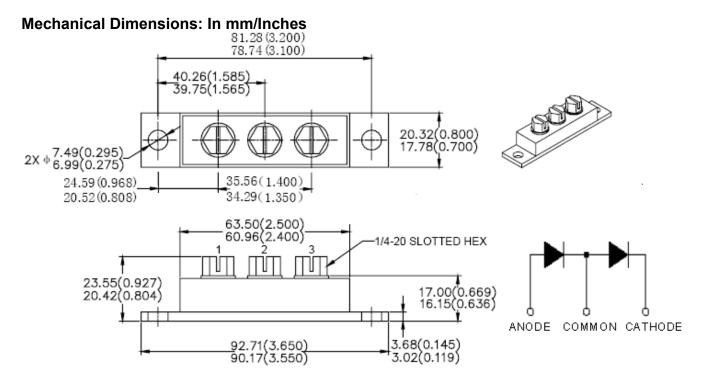
Please Note: Anode 1 = Terminal 1; Anode 2 = Terminal 3; Common Cathode = Terminal 2 Suffix R Denotes for Reversed Polarity.
